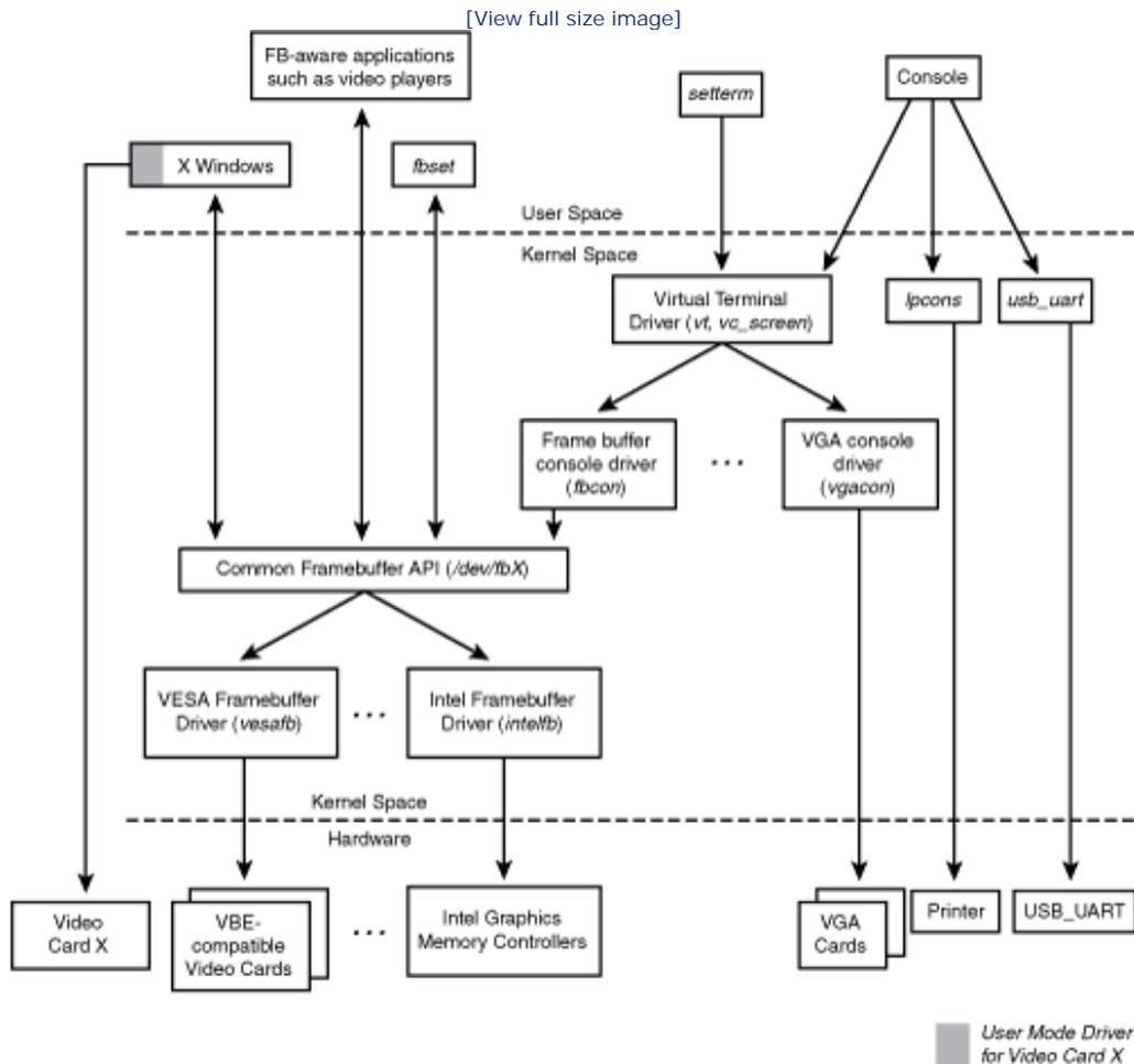
The Linux-Video subsystem shown in [Figure 12.5](#) is a collection of low-level display drivers, middle-level frame buffer and console layers, a high-level virtual terminal driver, user mode drivers part of X Windows, and utilities to configure display parameters. Let's trace the figure top down:
