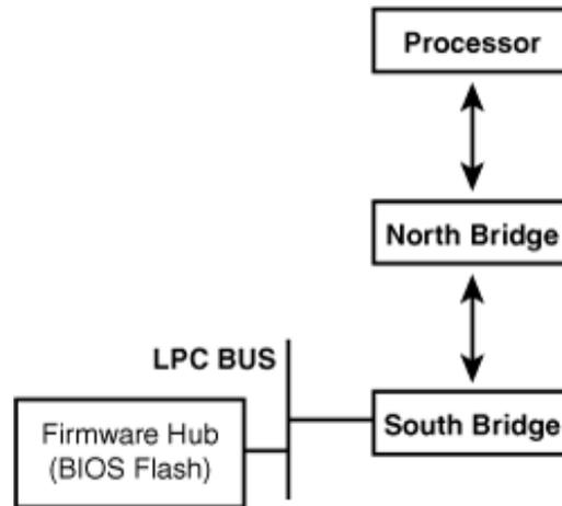
The MTD subsystem includes drivers to interface the processor with the FWH. FWBs are usually not compliant with the CFI specification. Instead, they conform to the JEDEC (*Joint Electron Device Engineering Council*) standard. To inform MTD about a yet unsupported JEDEC chip, add an entry to the `jedec_table` array in `drivers/mtd/chips/jedec_probe.c` with information such as the chip manufacturer ID and the command-set ID. Here is an example:
