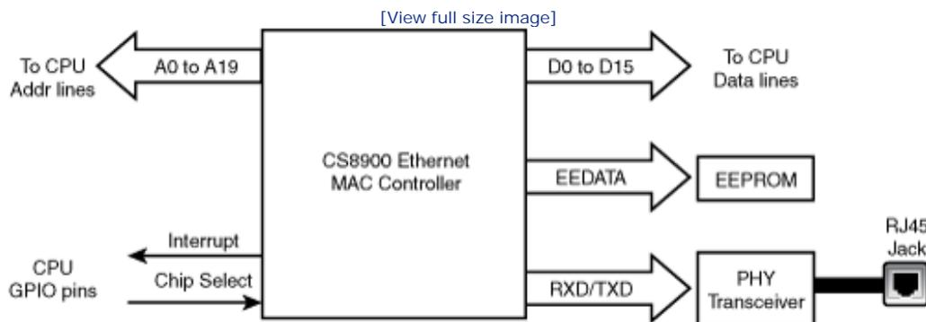
Look at `drivers/net/cs89x0.c` for the source code of the CS8900 driver. `cs89x0_probe1()` probes I/O address ranges to sense a CS8900. It then reads the current configuration of the chip. During this step, it accesses the CS8900's companion EEPROM and gleans the controller's MAC address. Like the driver in Listing 15.1, `cs89x0.c` is also built using `netif_*` and `skb_*` interface routines.
