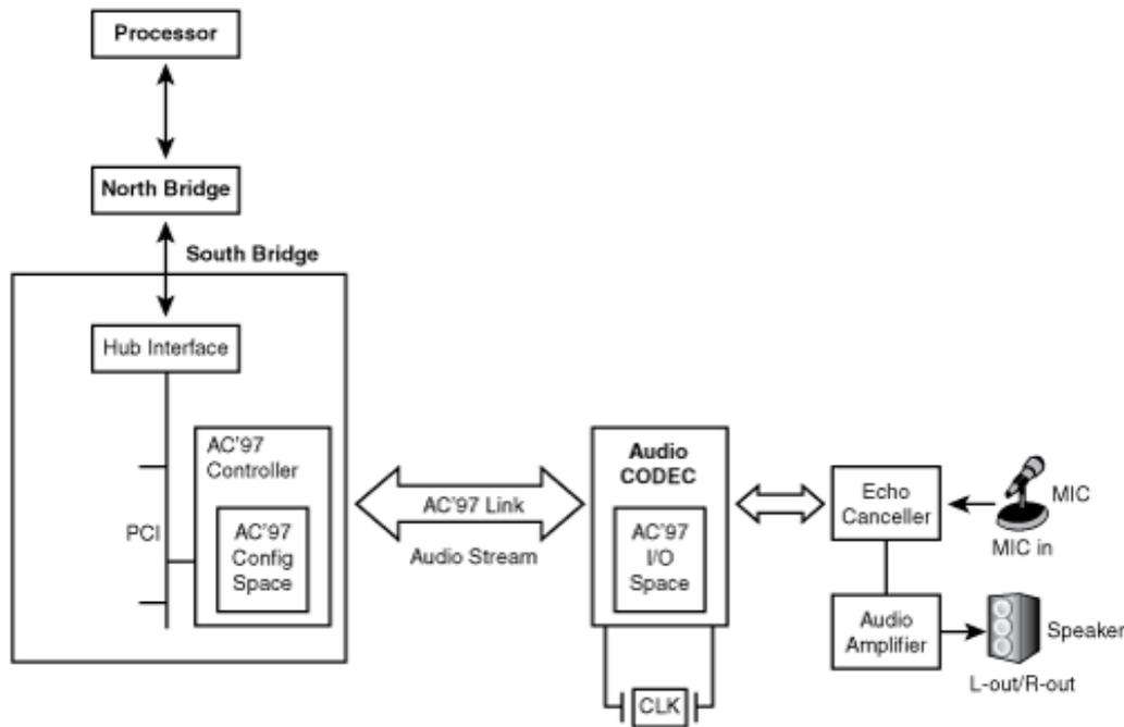
An *audio codec* converts digital audio data to analog sound signals for playing through speakers and performs the reverse operation for recording through a microphone. Other common audio inputs and outputs that interface with a codec include headsets, earphones, handsets, hands-free, line-in, and line-out. A codec also offers *mixer* functionality that connects it to a combination of these audio inputs and outputs, and controls the volume gain of associated audio signals.<sup>[1]</sup>
