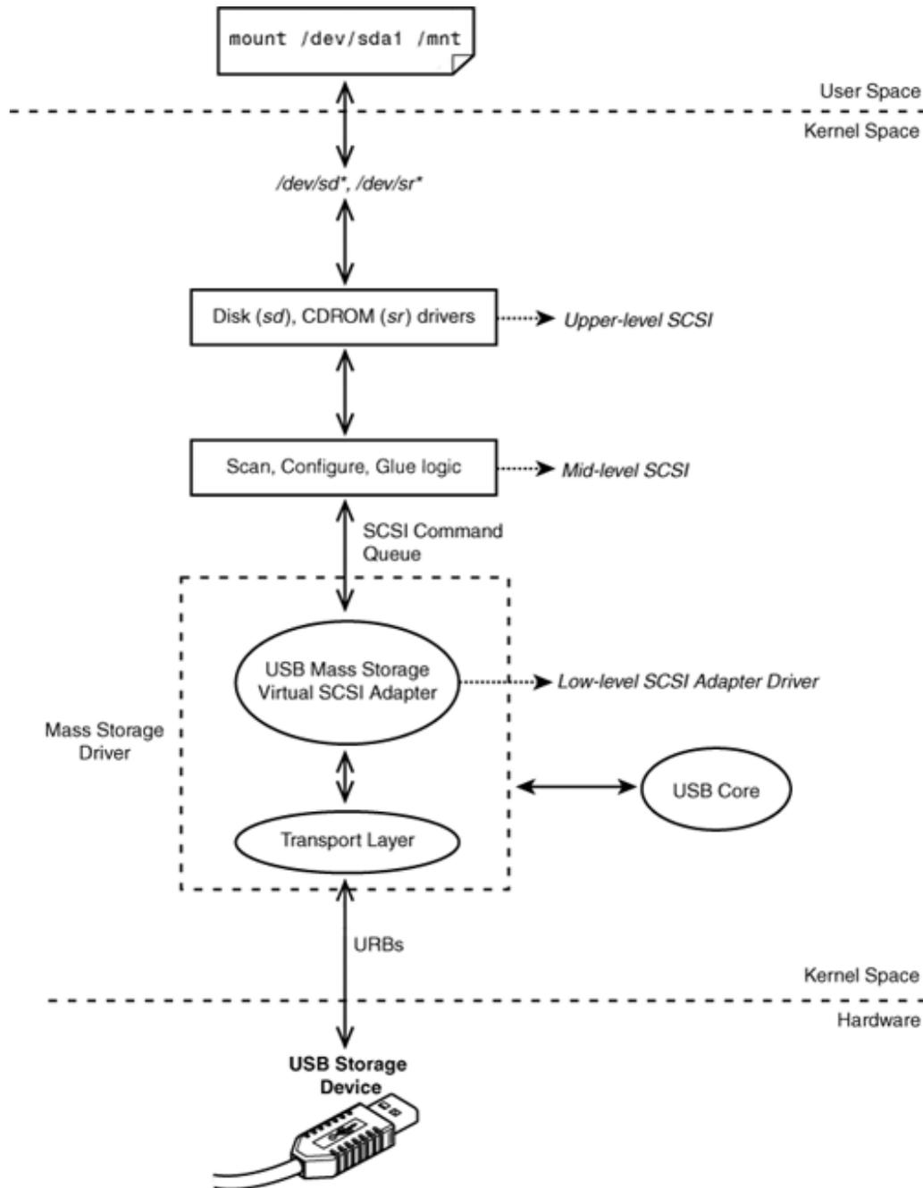
The mass storage driver registers itself as a virtual SCSI adapter. The virtual adapter communicates upstream via SCSI commands and downstream using URBs. A USB disk appears to higher layers as a SCSI device attached to this virtual adapter.
