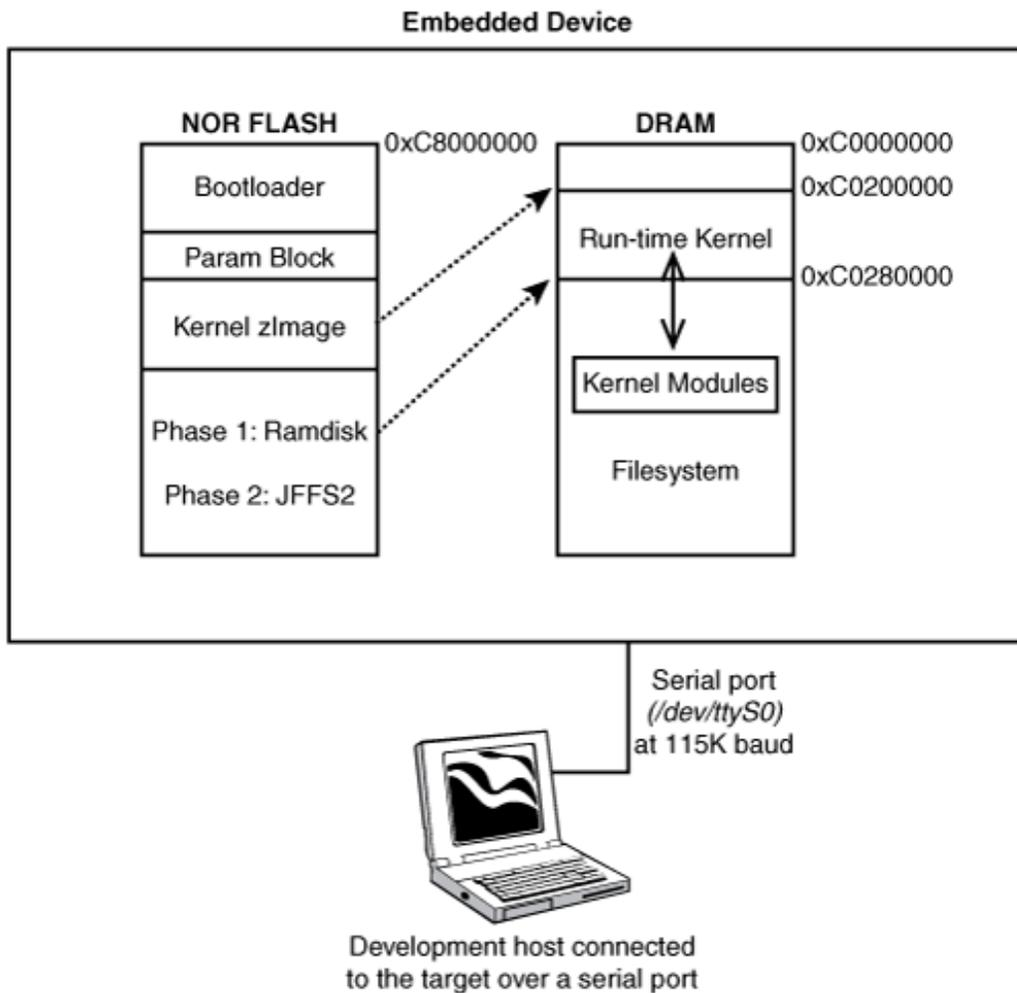
During power-on, the bootloader in Figure 18.2 uncompresses the kernel and loads it to DRAM at 0xc0200000. It then loads the ramdisk at 0xc0280000 (unless you build an *initramfs* into the base kernel as you learned in Chapter 2). Finally, it obtains command-line arguments from the *param* block and transfers control to the kernel.
