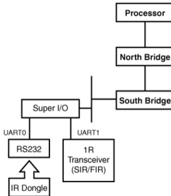
Figure 16.5. IrDA on an embedded device (for example, EP7211).
