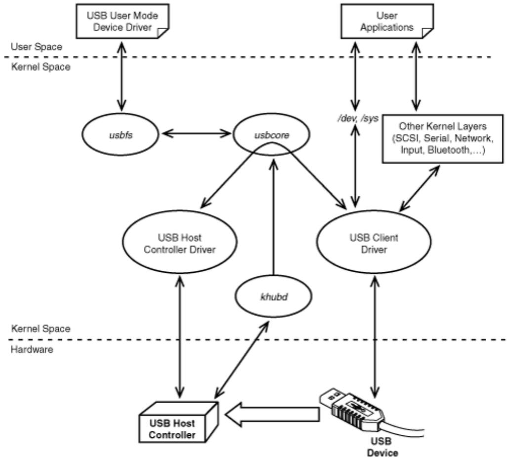
For end-to-end operation, the USB subsystem calls on various other kernel layers for assistance. To support USB mass storage devices, for example, the USB subsystem works in tandem with SCSI drivers, as shown in [Figure 11.3](#). To drive USB-Bluetooth keyboards, the stakeholders are fourfold: the USB subsystem, the Bluetooth layer, the input subsystem, and the tty layer.
