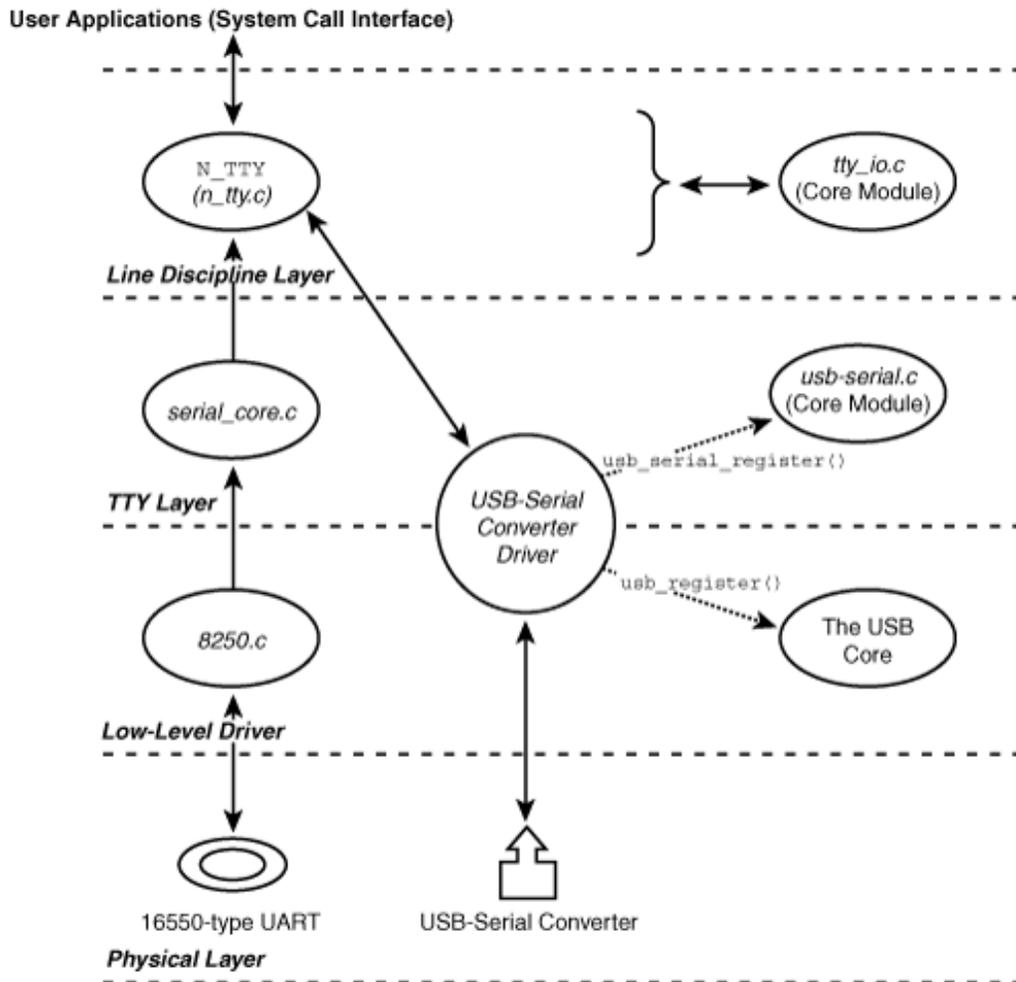
A USB-serial driver is similar to other USB client drivers except that it avails the services of a USB-Serial core in addition to the USB core. The USB-Serial core provides the following:
