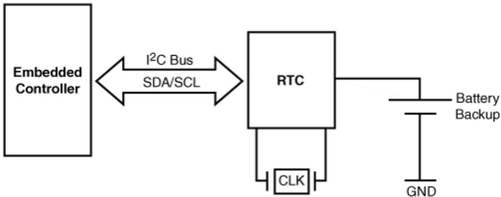
Assume that the I<sup>2</sup>C slave address of the RTC is `0x60` and that its register space is organized as shown in [Table 8.2](#).
