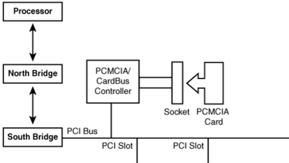
Figure 9.2. PCMCIA on an embedded system.
